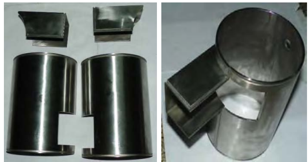
Fig.14: Assembled water cooling jacket with welding lip.
