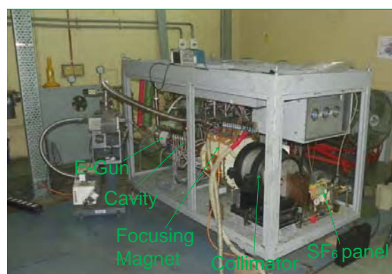
Fig. 1: 6 MeV compact linac.
