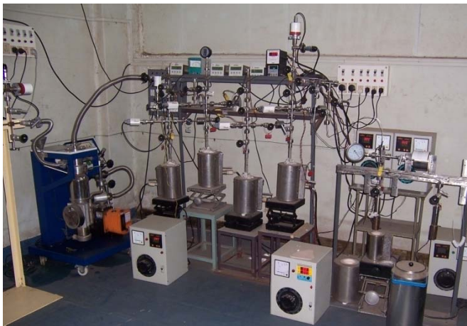
Fig. 1: Indigenously designed Sieverts' type volumetric apparatus.
