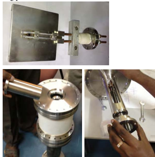
Fig.4: Shrink fitting of two Copper pin feed through with Invar connector and alignment fixture.
