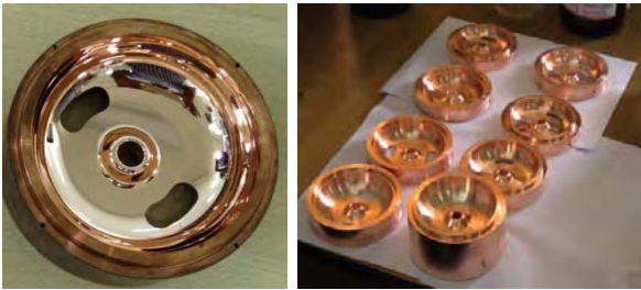
Fig.16: Internal Diamond turned cavity.
