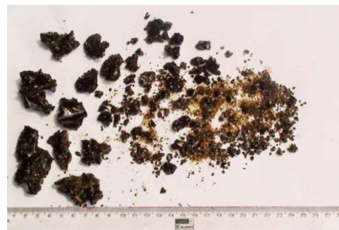
Fig. 19 c: Experimental demonstration of quenching of melt stimulant
