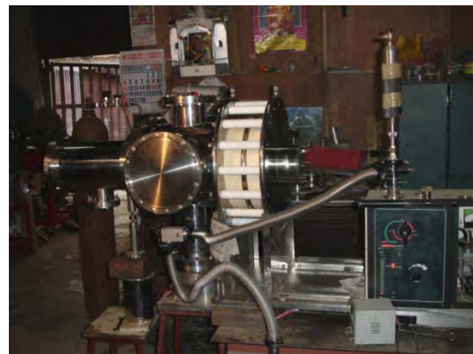
Fig: 21: ECR Ion source under leak testing
