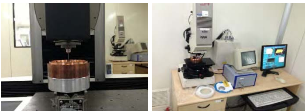
Fig. 19: Co-ordinate measurement of cavity and surface roughness measurement by white light interferometer.
