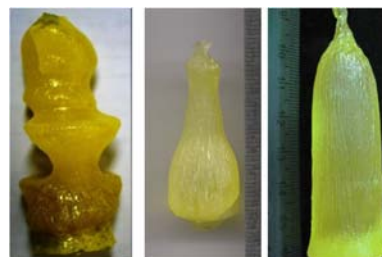
Fig. 1: The photograph of GGAG:Ce crystals as grown in an initial run and after optimizing the growth parameters.
