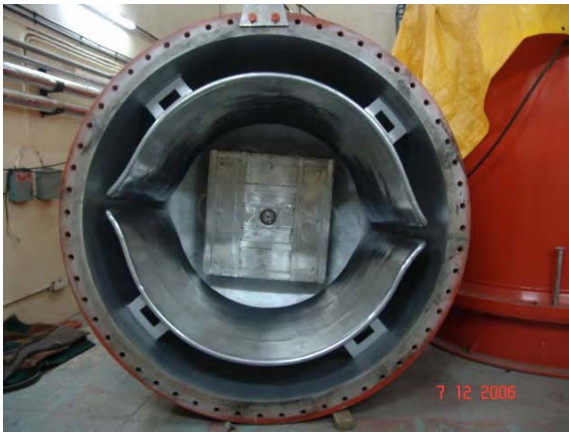
Fig.11: Rectangular Radiator Type Heat Exchanger inside the Accelerator Tank.
