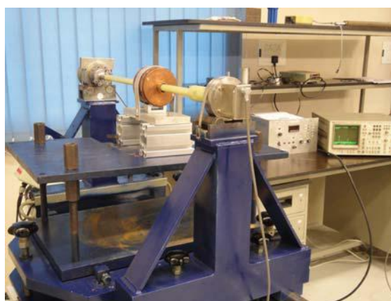
Fig 10(b): PMQs being measured at Harmonic Coil Magnetometer at RRCAT (Measurements & Photo courtesy : AMTD, RRCAT)
