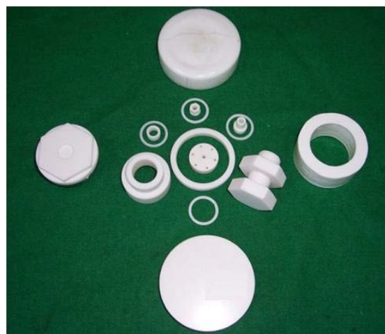
Various components fabricated from machineable MAS glass-ceramics
