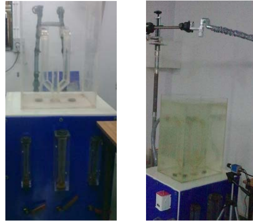
(a) Set up for PIV stud (b) Arrangement for Laser and Camera Fig. 9: Experimental Setup for flow mixing study
