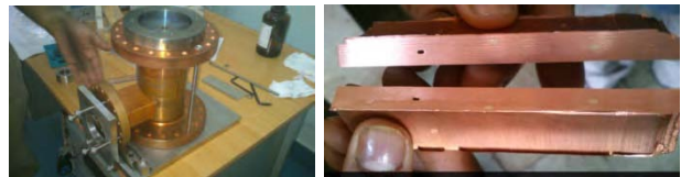
Fig. 13: ETP Copper brazed cavity sample for tensile test.
