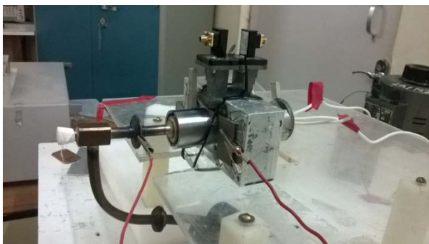
Fig. 7. Prototype miniature klystron tube integrated with developed magnet assembly
