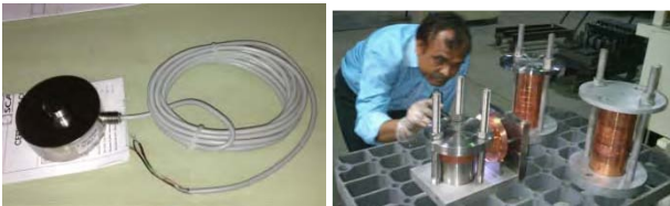
Fig.18: Load Cell for 2.5 ton load and assembled cavity before brazing.
