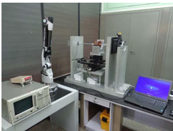
Fig 10(a): PMQs being measured on Hall Probe Magnetometer at BARC
