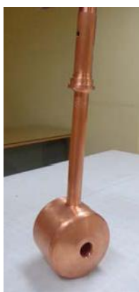
Fig 9: Snap shot of developed Drift Tube with embedded PMQ
