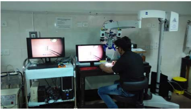
Fig. 4: The Trimiti system running active and passive stereoscopic vision using surgical microscope.
