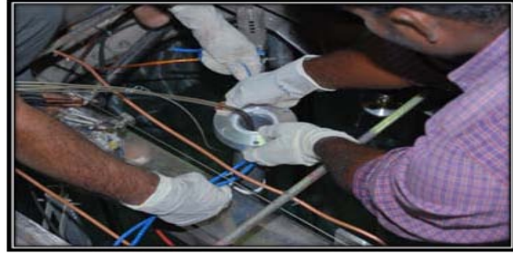
Fig.8 Calibration Facility at KAMINI reactor being used for testing of neutron detectors
