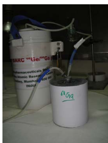
'BARC' ^{68}\text{Ge}/^{68}\text{Ga} generator
