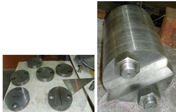
Fig. 7: Assembly of collimator plates with alignment gauge.
